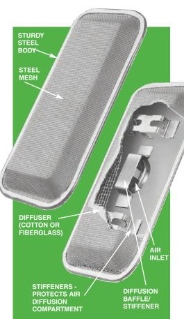
Exclusive new heavy-duty construction features stiffeners to prevent crushing of air compartment. These stiffeners eliminate the possibility of the Aerator being crushed by a head of material or by a man stepping on it when cleaning bin. The stiffeners do not obstruct the diffusion of air.
